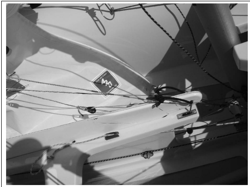
Electric tape trim lines and lines on the board to gauge depth.
