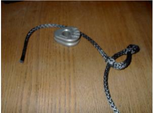
Next up, take the second inside out hole and un-invert it like the first one but this time by pulling out the tail side of the rope
