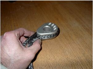
Now, wrap the rope around the thimble, starting from the inside out hole, to form your loop. It is important that you do not wrap the tail around the part but the other side of the rope; the longer side. Tighten it nicely and mark the other side of the rope where it meets with the inside out hole.
