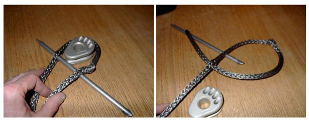
Again, open the braid with a splicing fid where you just marked it. \* (see note 2 and 3 at the top of the 1st
