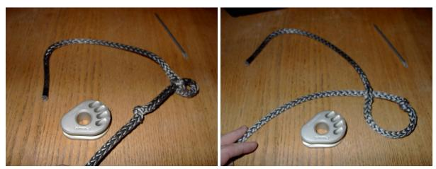
Next up, take the first inside out hole (the one closest to the tail's end) and un-invert it by pulling out the longer side of the rope (not the tail side of it)
