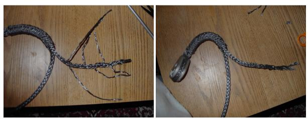
Here is the most important part of it, the tapering of the tail. Unbraid strands from the tail and cut them to varying length to form a perfect taper. For example, if you work with a 12 strand rope and your tail is 480mm long, divide 480 by 12 and cut a strand every 40mm.
