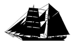
**Brigantine**, a two masted vessel square rigged on the foremast, with fore-and-aft sails on the mainmast. The drawing shows a typical Bluenose softwood vessel of about 220 tons, similar to the Spencers Island built Amazon which later became the famous mystery ship Mary Celeste. The brigantine is shown with two staysails set between the masts.
