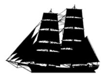
**Brig**, a two masted vessel square rigged on both masts. The brig is a very old and efficient sailing rig, and the class was still in use up to the very end of commercial sailing ships. Only a few brigs were built in Nova Scotia yards, but they were very common in European waters.
