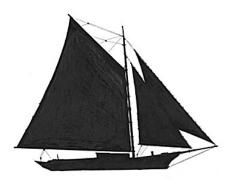
**Sloop** A fore and aft rigged vessel with one mast is a sloop. In the early 1800s some large sloops traded with the West Indies, but most sloops in the 19th century were small inshore fishing vessels. In the 20th century, sloops became the most popular rig for yachts.
