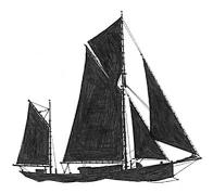
**Ketch** A two masted sailing vessel where the mizzen mast is ahead of the rudder. The rig is similar to a schooner but the main mast (the tallest mast) is the first mast, not the second mast. Ketches were common in 19th century Europe but rare in Nova Scotia until they became very popular for yachts in the 20th century.
