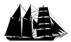
**Barquentine**, a vessel with the foremast rigged square, and the other masts rigged fore and aft. Our vessel is similar to the Maid of England of 750 tons built at Grosses Coques in 1919. She was the last Canadian commercial vessel to carry a square rig, being abandoned at sea in 1928. Only a small number of this type were built locally.
